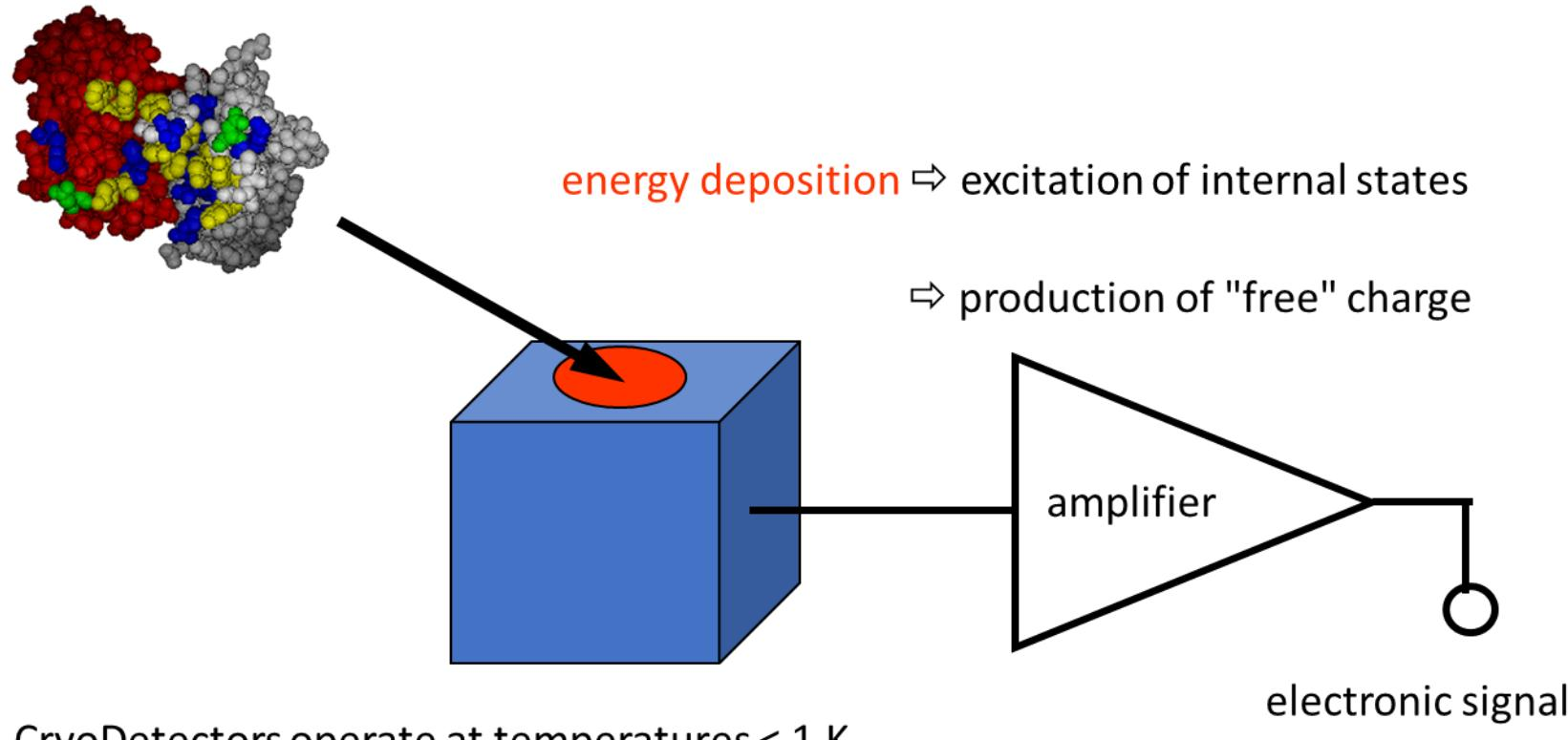
CryoDetectors operate at temperatures < 1 K
