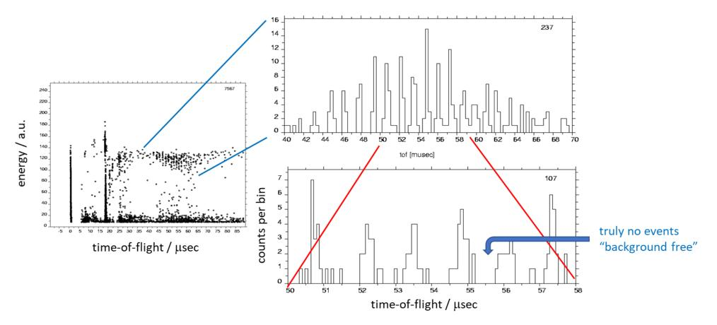
Polystyrene 2000: varying laser power induces different fragmentation patterns. For the same time-of-flight (mass) the molecule has different kinetic energies (details are not yet understood, but may provide information about MALDI process)
